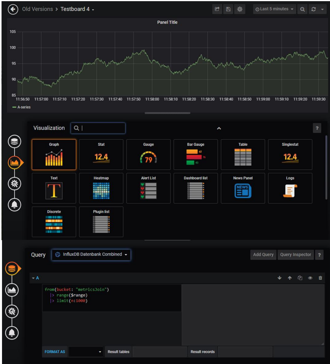
Figure 24. Exemplary representation of the possible visualizations of data in a dashboard panel
