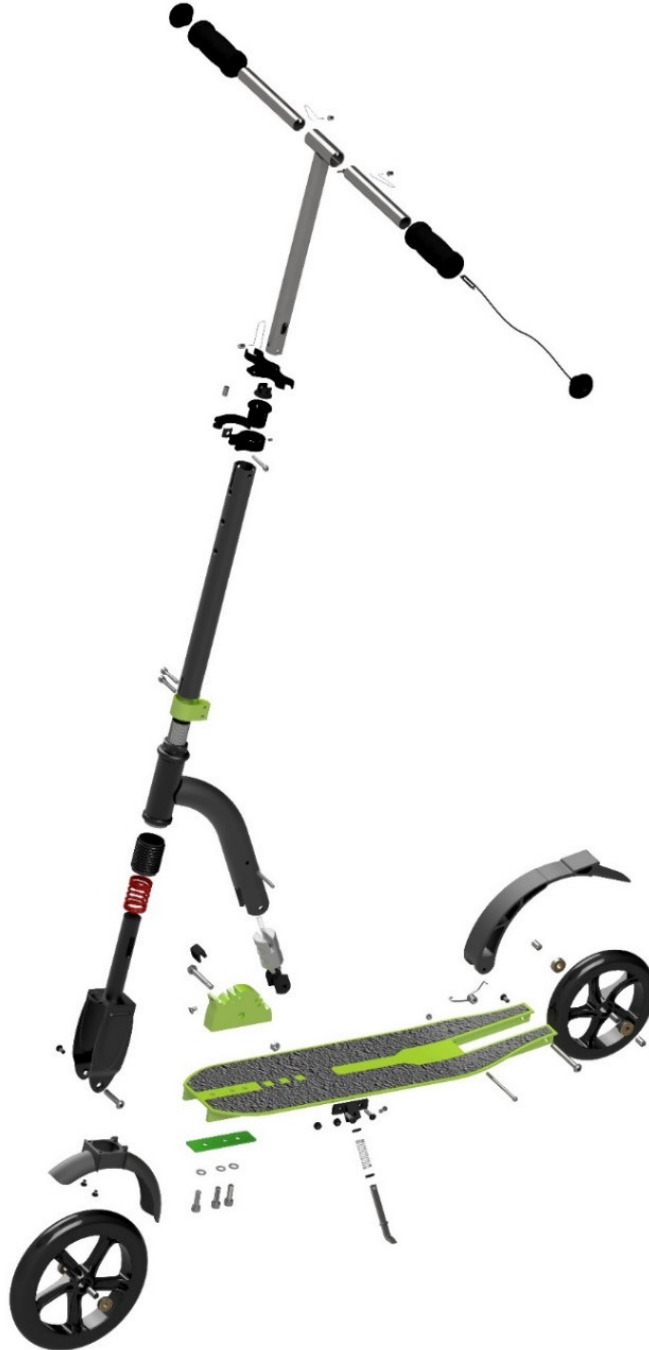
Figure 2. Exploded view of the scooter, assembled in the LEAD Factory
